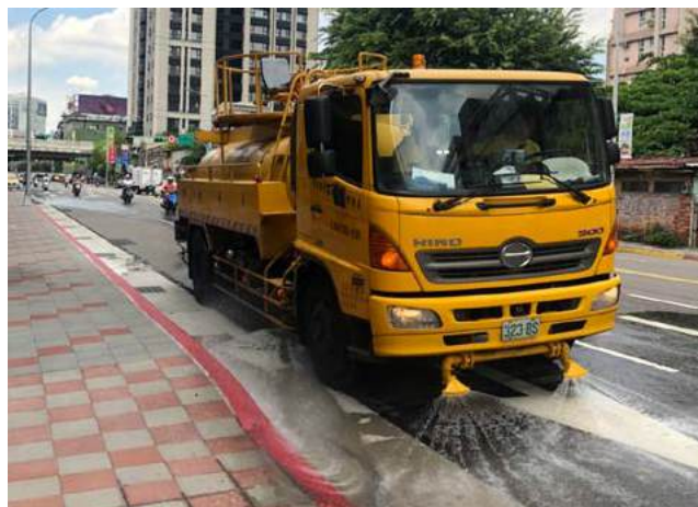
► Water sprinkling to lower temperature on the surface of the roads.
