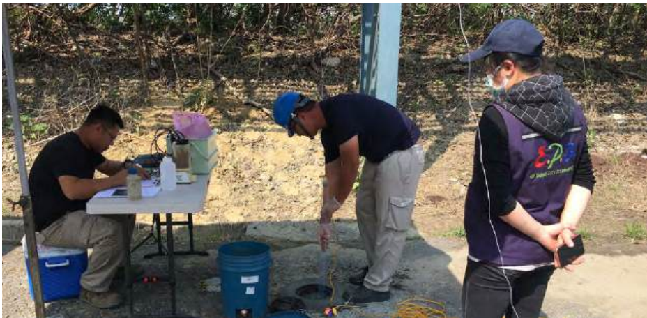
△ Groundwater Monitoring by Monitoring Wells in Industrial Areas
